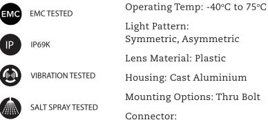
Light Pattern: Symmetric, Asymmetric Lens Material: Plastic Housing: Cast Aluminium Mounting Options: Thru Bolt Deutsch (DT04-2P) built in
