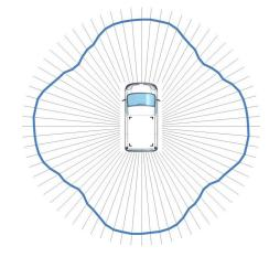
4 Corner Module LEDs fitted on the corners of a vehicle produce a stong homogeneous 360° warning signal as shown in the diagram.
